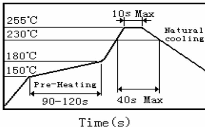
(2) 烙铁焊接 Soldering Iron
