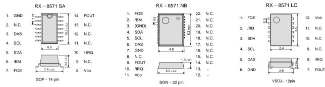
The metal case inside of the molding compound may be exposed on the top or bottom of this product. This purely cosmetic and does not have any effect on quality, reliability or electrical specs.
