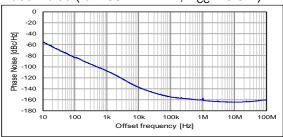
Phase Jitter (12 kHz to 20 MHz): 19 fs Typ.
