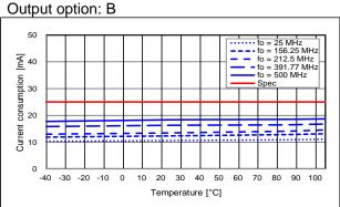
$V_{CC}$  = 2.5 V, Temperature Characteristic
